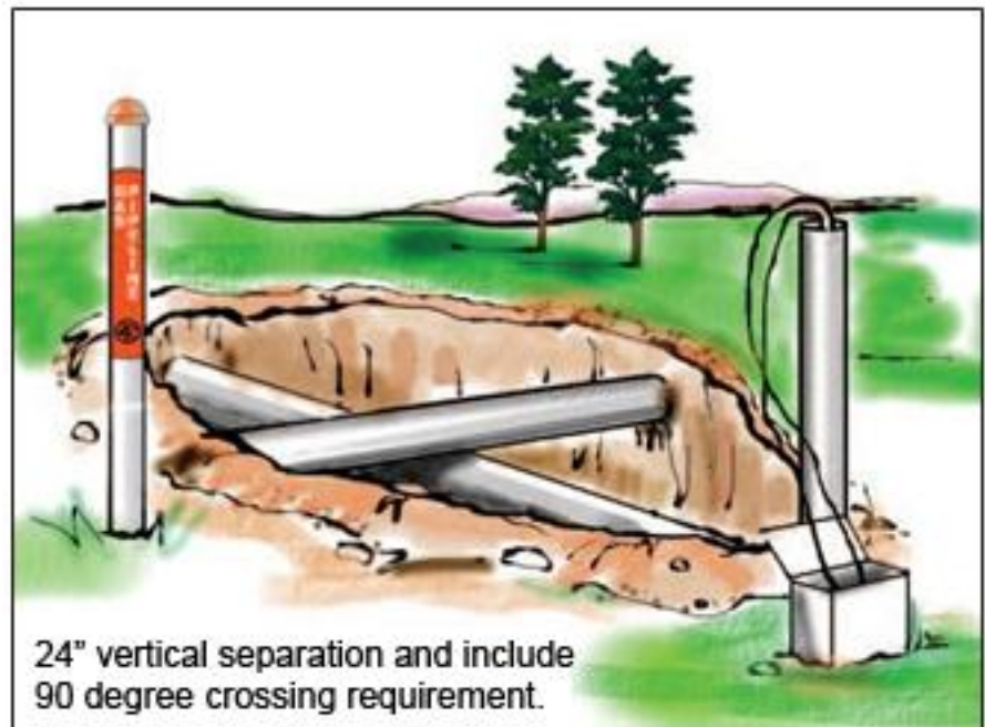
FIGURE 2: DOT-APPROVED PIPELINE MARKERS, CATHODIC PROTECTION BONDS, AND POTENTIAL LEADS ARE AT ALL CROSSINGS AND TERMINATE AT ABOVE-GROUND LOCATIONS.
